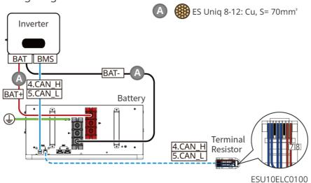
GW14.3-BAT-LV-G10: When the battery is directly connected to two 1-way output inverters, the wiring diagram is as follows:
