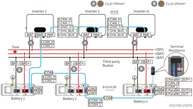
GW14.3-BAT-LV-G10: When the battery is directly connected to a single 1-way output inverter, the wiring diagram is as follows:
