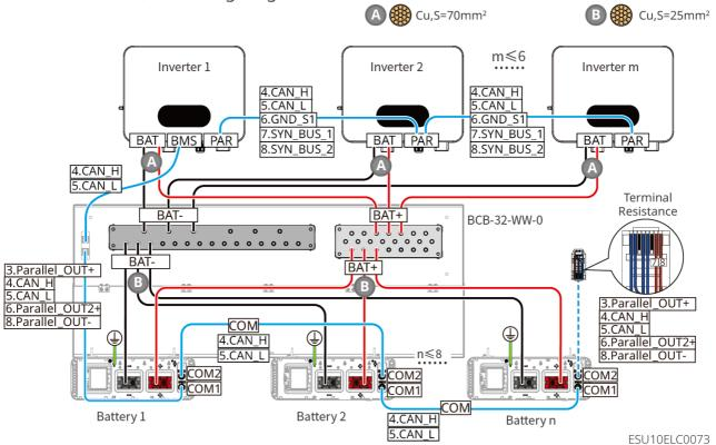
LX U5.0-30: When the battery quantity is less than or equal to 15, and the busbar BCB-33-WW-0 is used, the wiring diagram is as follows:
