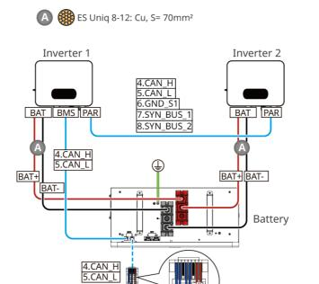
GW14.3-BAT-LV-G10: When the battery is in hand-to-hand connection with a single 1-way output inverter, the wiring diagram is as follows:
