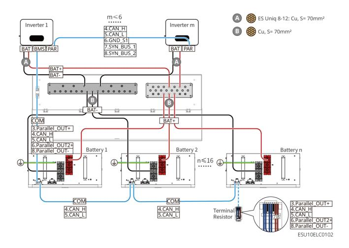
GW14.3-BAT-LV-G10: When the number of batteries is less than or equal to 16 and a third-party busbar is used to connect to 1-way output inverter, the wiring diagram is as follows:
