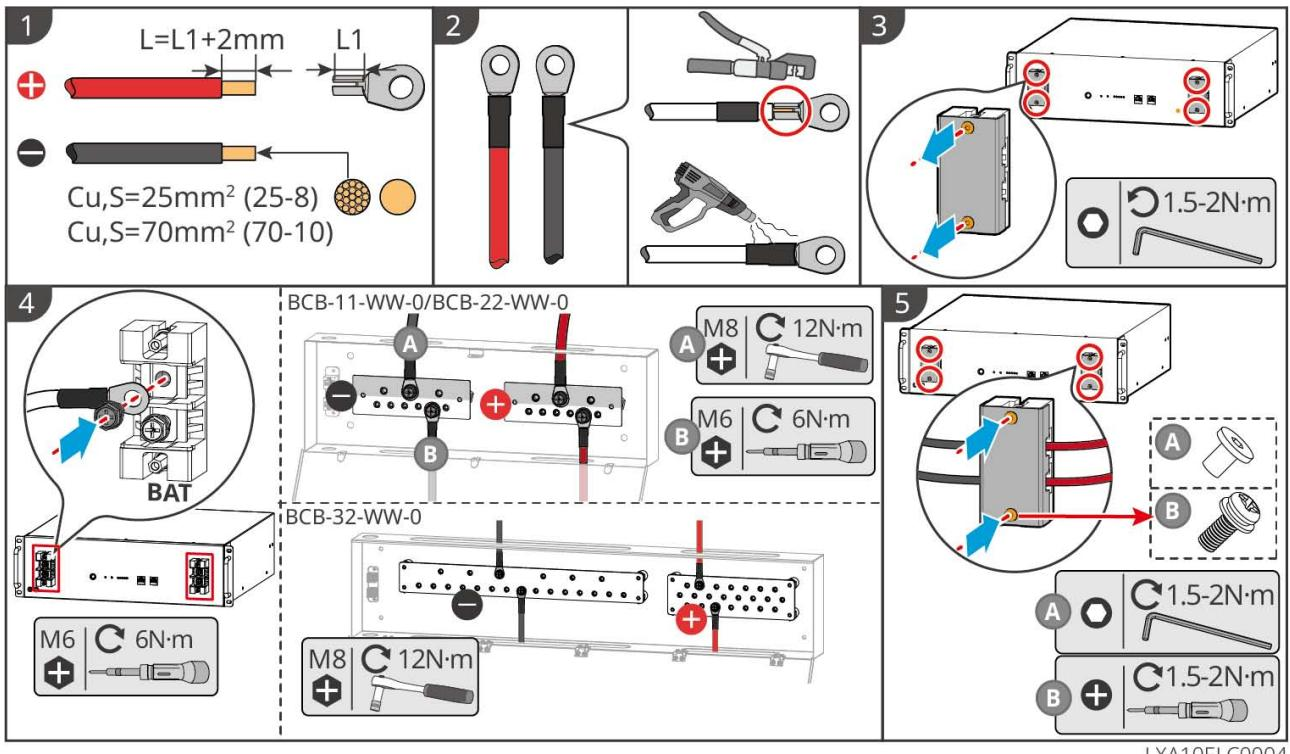
Terminal cable fabrication method (LX A5.0-30)
