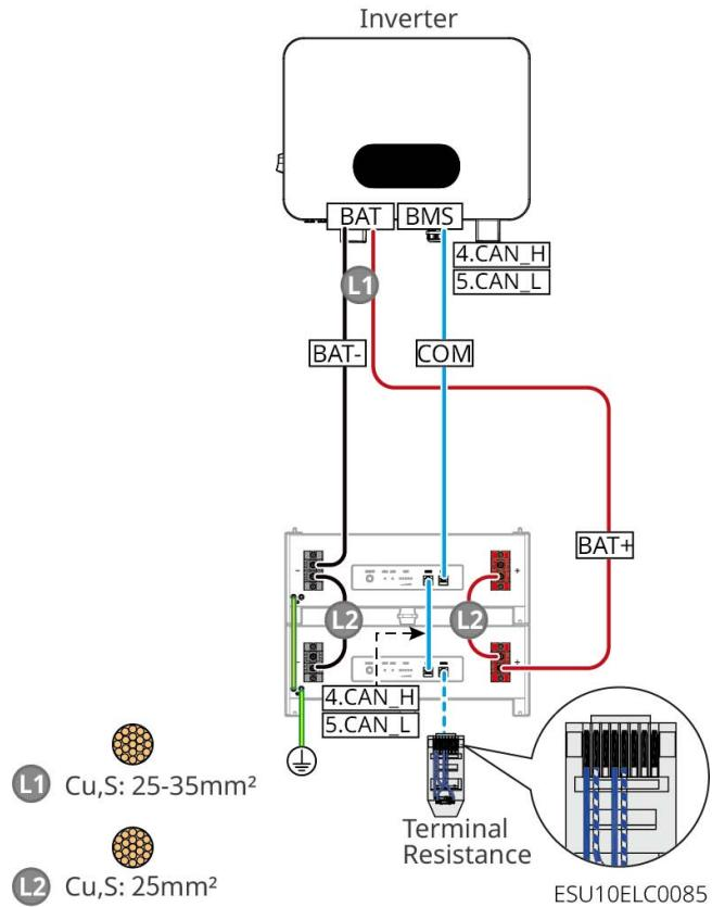
LX A5.0-10: Battery in conjunction with busbar BCB-11-WW-0 connection method
