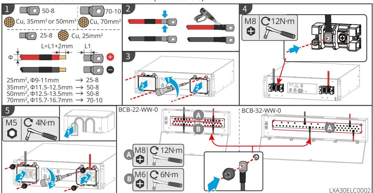
Cable termination method for Battery end (LX U5.0-30)
