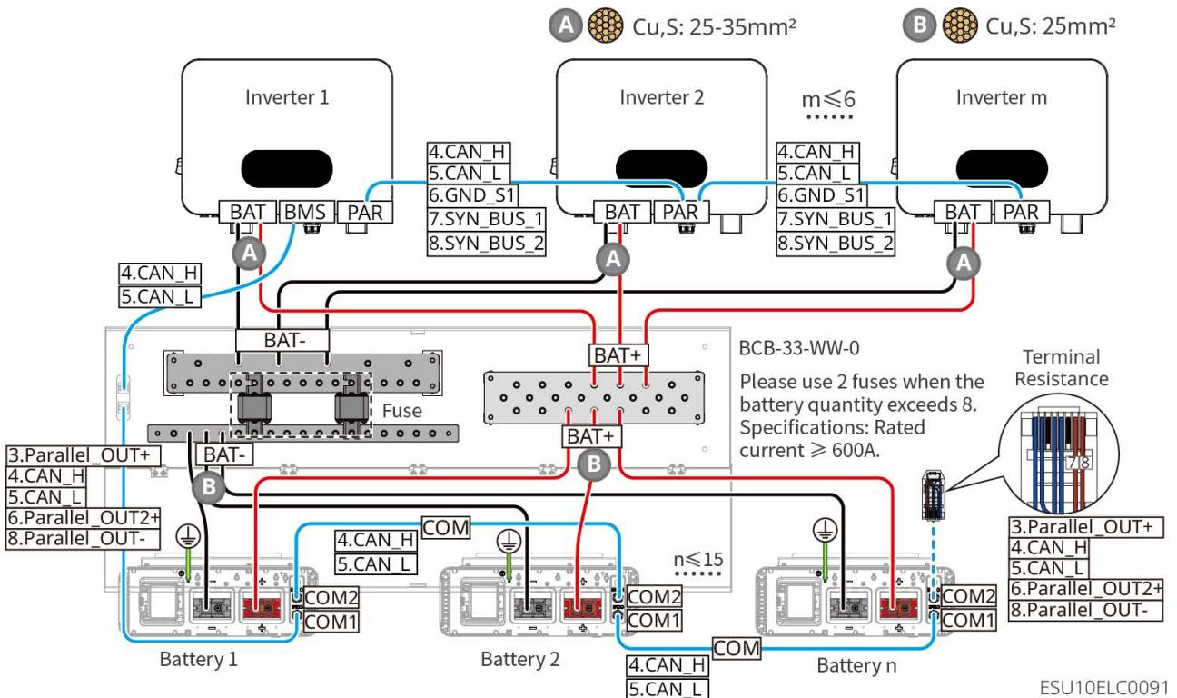
LX U5.0-30: When the number of Battery  $\leq 8$ , Battery is paired with a third-party combiner box connection method.
