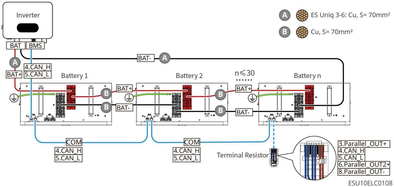
GW14.3-BAT-LV-G10: When the number of Battery is less than or equal to 15, and a busbar (BCB-32-WW-0, current ≤ 720A) is used to connect one output Inverter, the wiring diagram is as follows:
