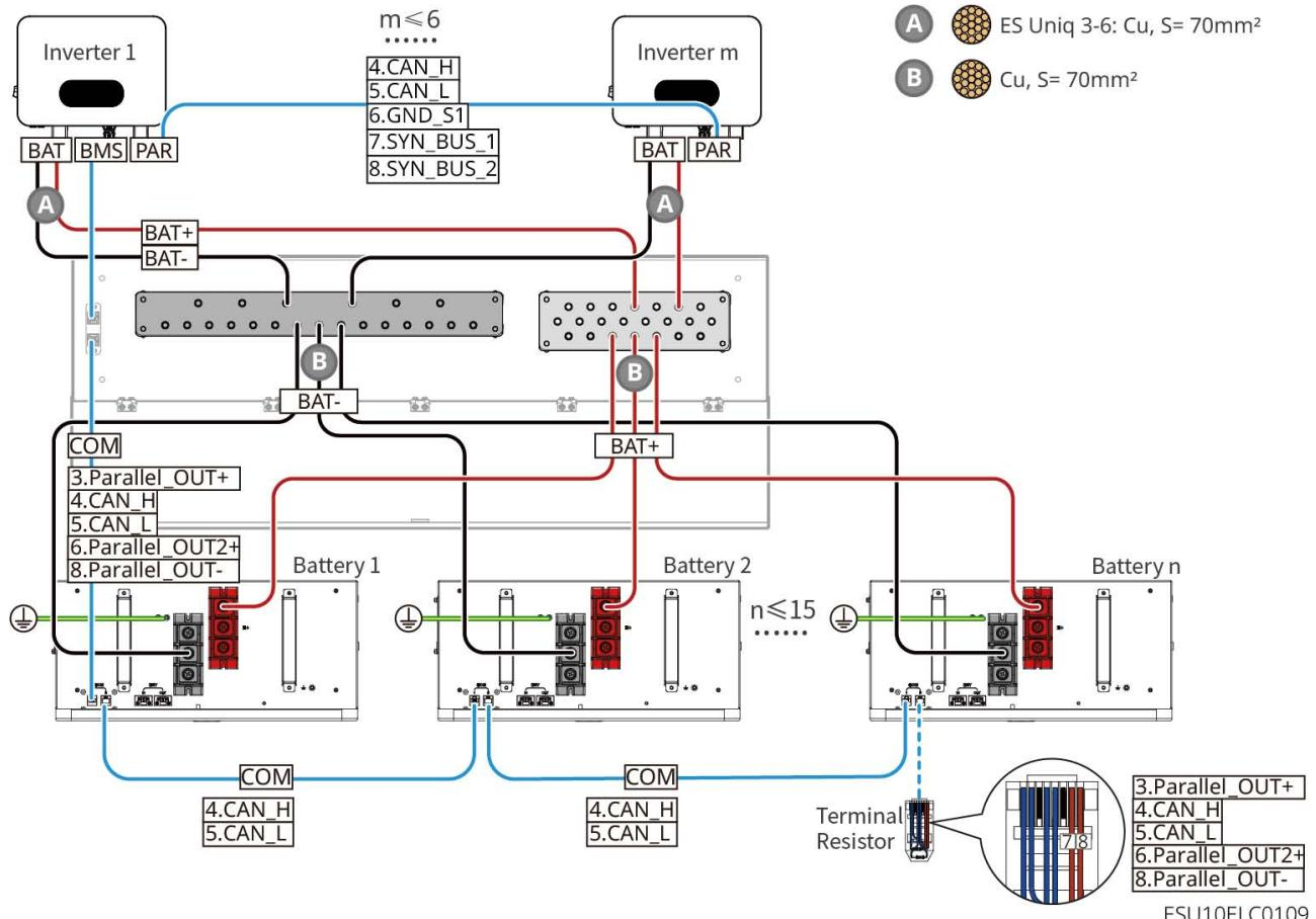
GW14.3-BAT-LV-G10: When the quantity of Battery is less than or equal to 30, and a third-party busbar is used to connect one output Inverter, the wiring diagram is as
