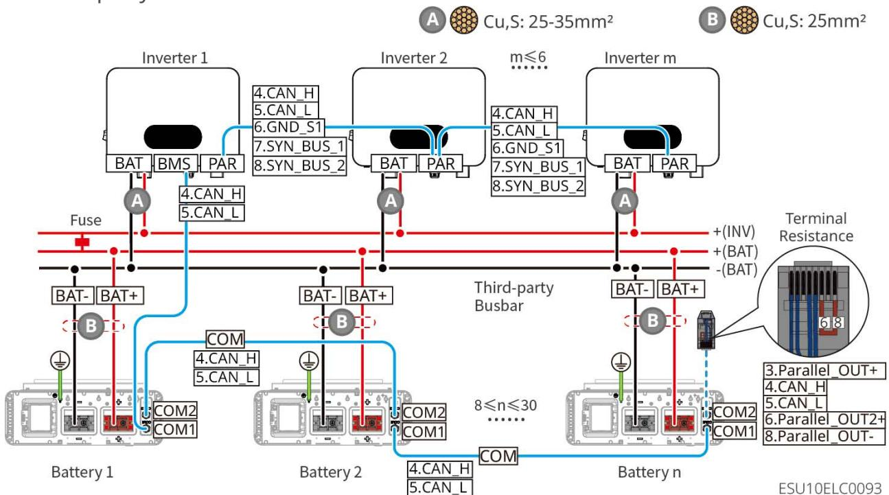
GW14.3-BAT-LV-G10: When Battery is directly connected to a single 1-channel output Inverter, the wiring diagram is as follows:
