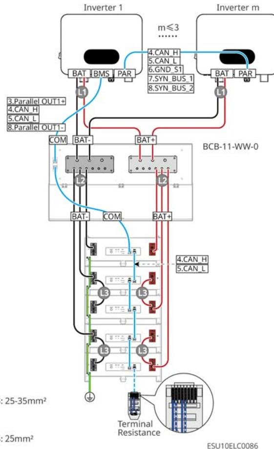
LX A5.0-10: Battery in conjunction with busbar BCB-22-WW-0 connection method
