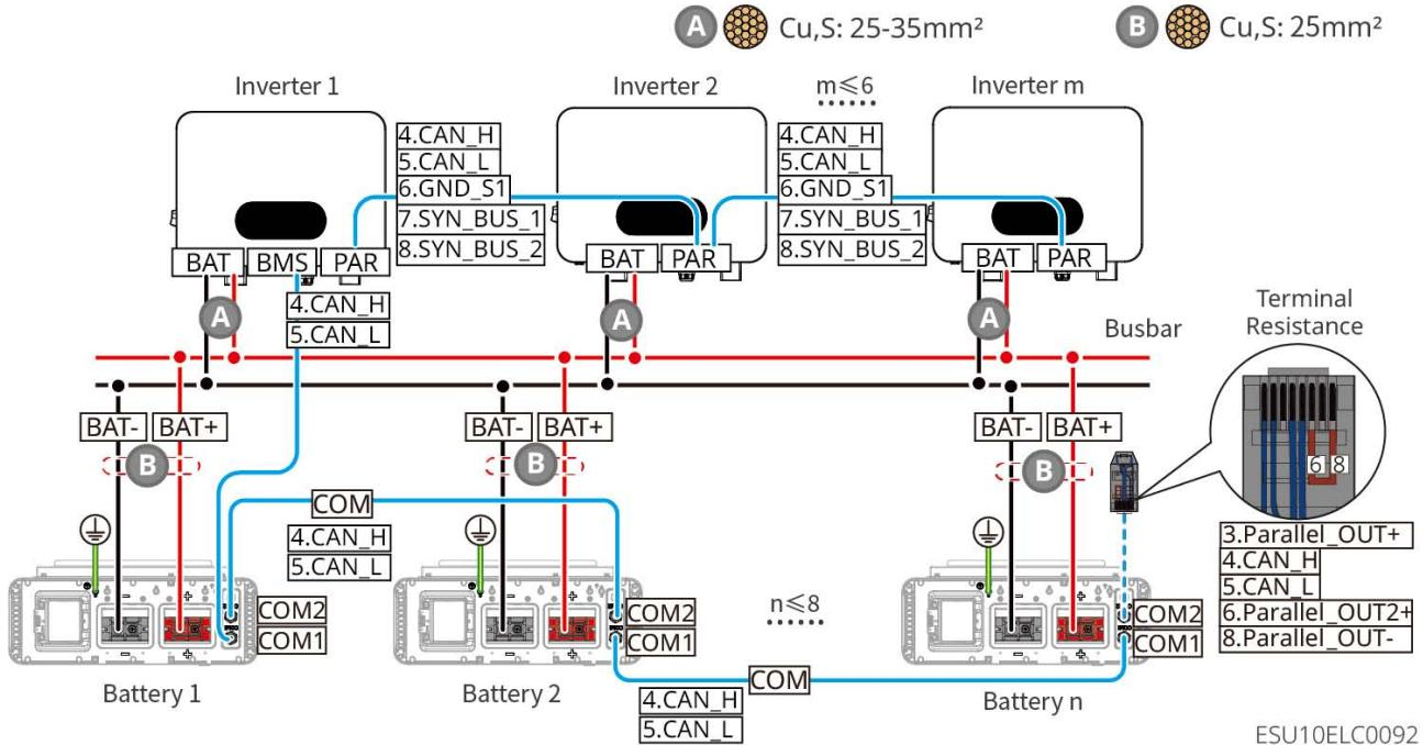
LX U5.0-30: When the number of Battery exceeds 8 units, Battery shall be connected via third-party busbar.
