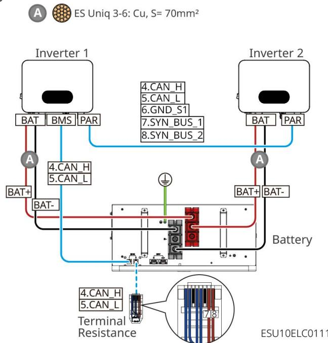
GW14.3-BAT-LV-G10: When Battery is connected in a daisy-chain configuration with a single 1-channel output Inverter, the wiring diagram is as follows:
