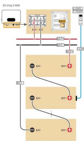
The quantity of batteries depends on the required voltage.
