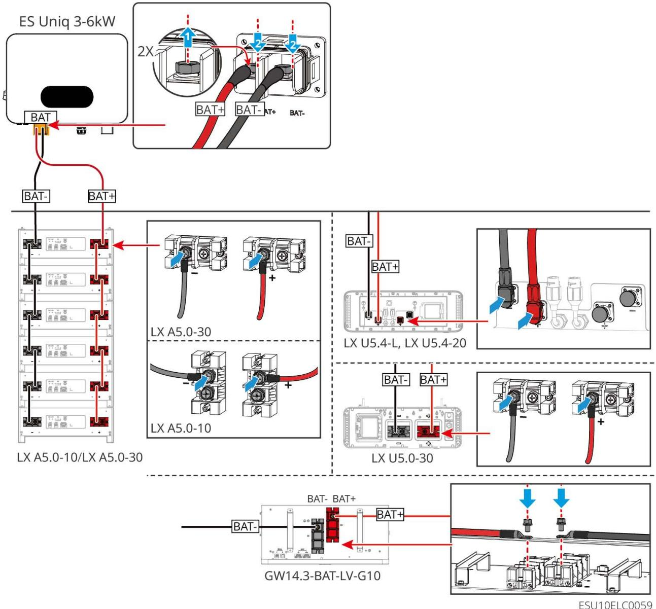
Inverter terminal cable fabrication
