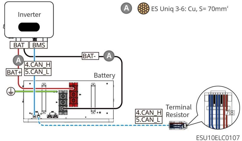
GW14.3-BAT-LV-G10: When Battery is directly connected to two single-output Inverter units, the wiring diagram is as follows:
