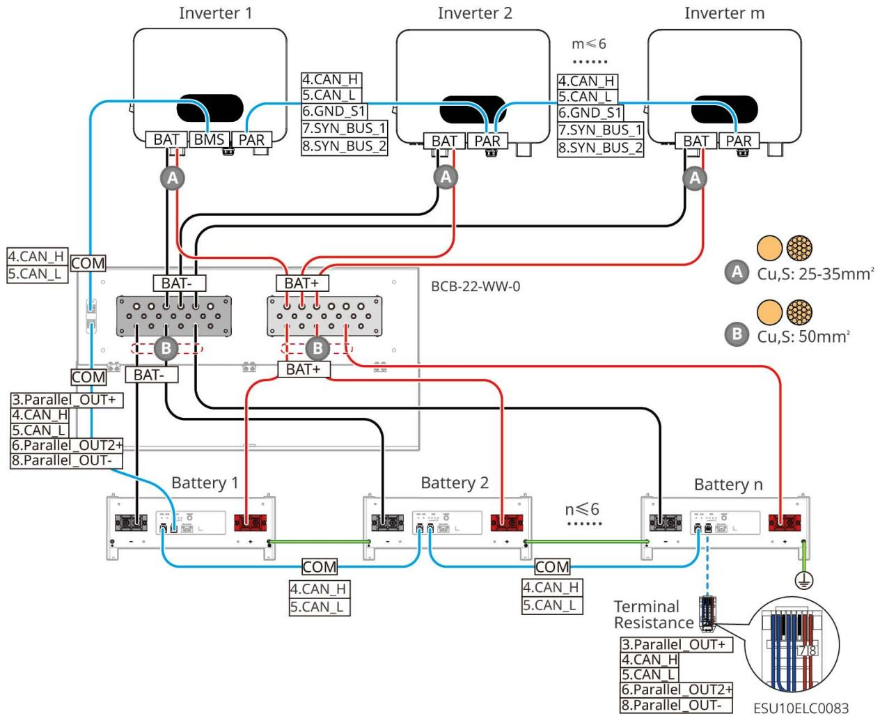
LXA5.0-30: Compatible with busbar BCB-32-WW-0 connection method
